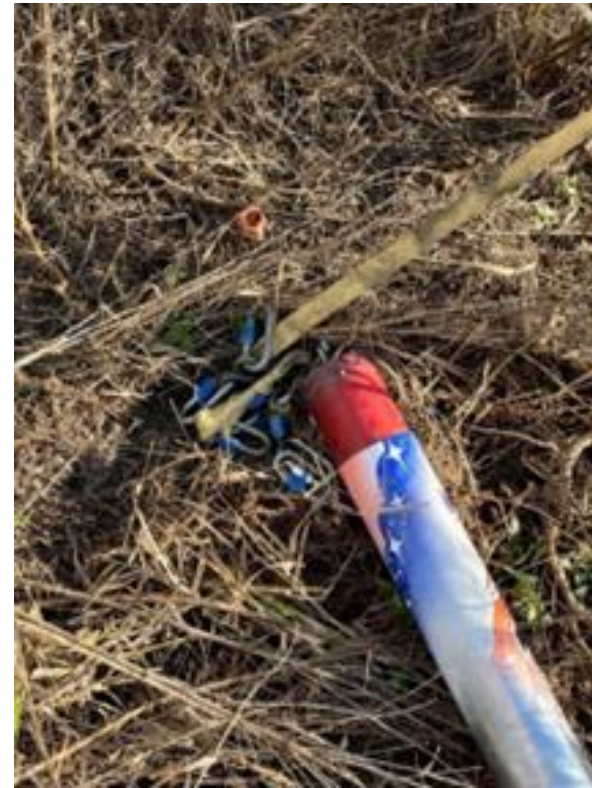
Recovery Harness and Ballasts Attached to the Aft Section
