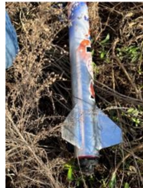
Aft Section of the Launch Vehicle with the Conditions of the Fins
