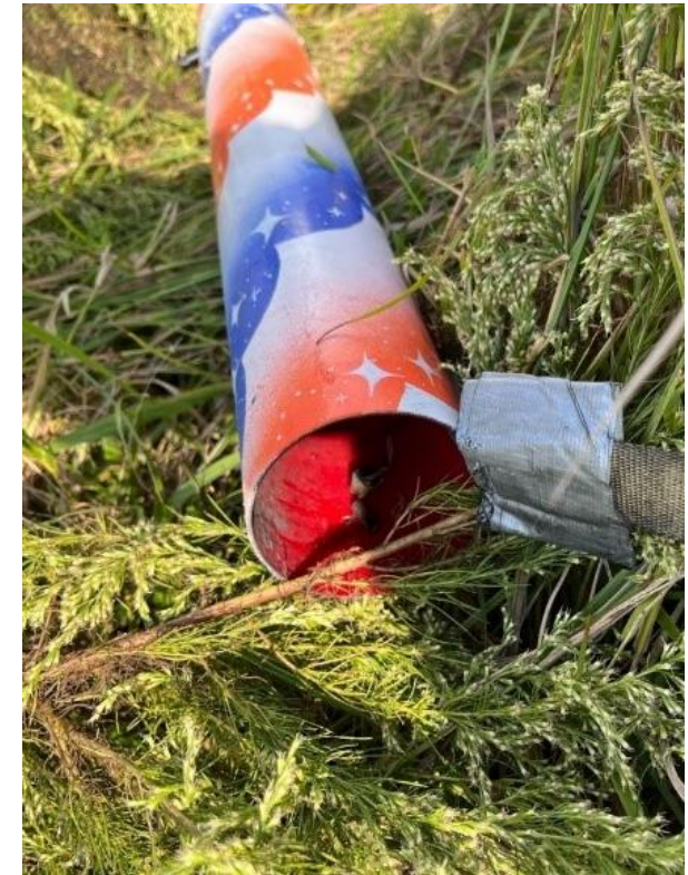
Recovery Harness which Connects the Forward and Central Sections
