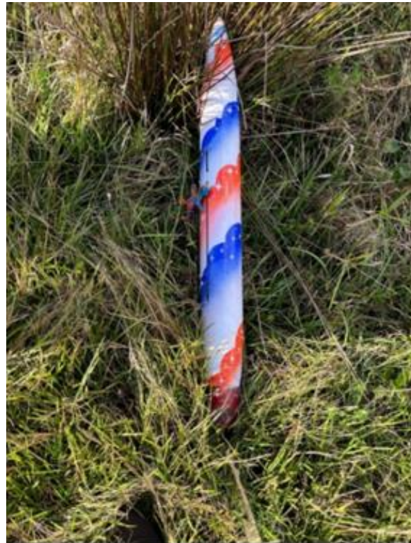
Nosecone with Payload Bay Door Still Intact
