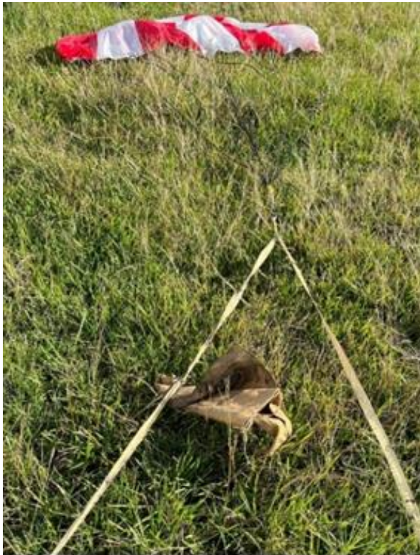
Fully Deployed Main Parachute with the Parachute Protector and Recovery Harness
