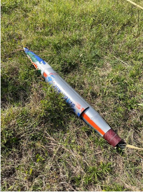
Figure 11: Payload Section Viewed From Aft with Unlocked Door
