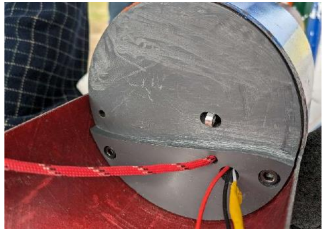
Figure 5: Payload Aft Bulkhead Showing Wires, Attached Recovery Harness, and Beam from Rack and Pinion Mechanism
