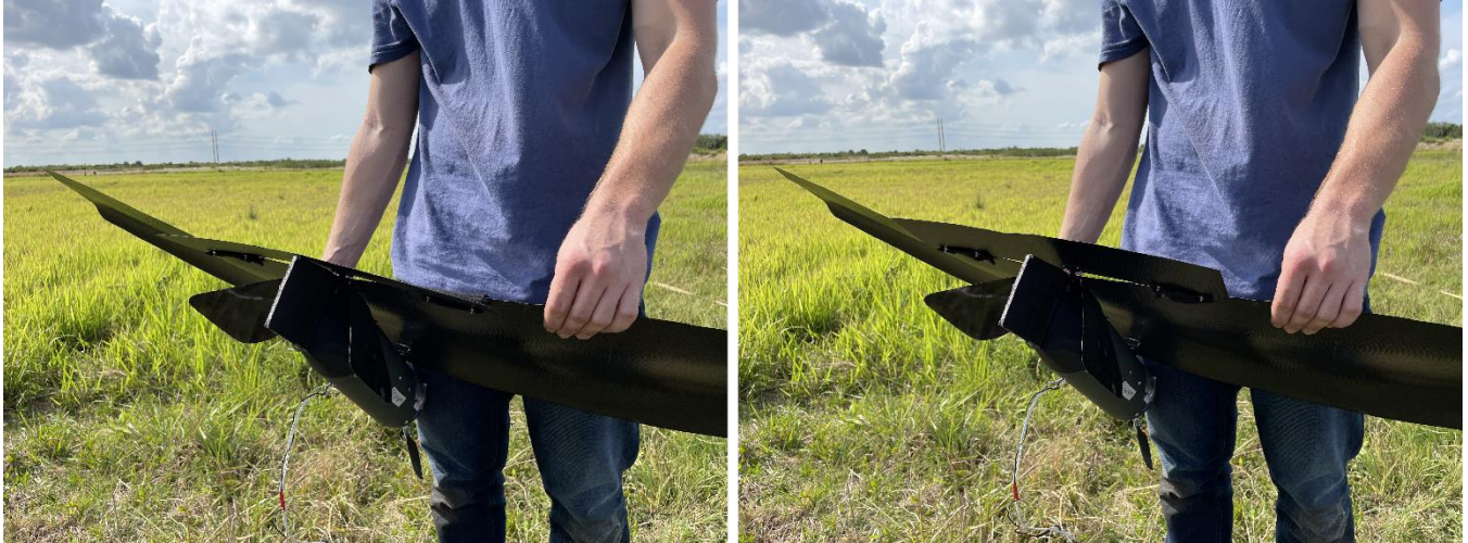
Figure 22: Demonstration of Elevator Function After Flight
