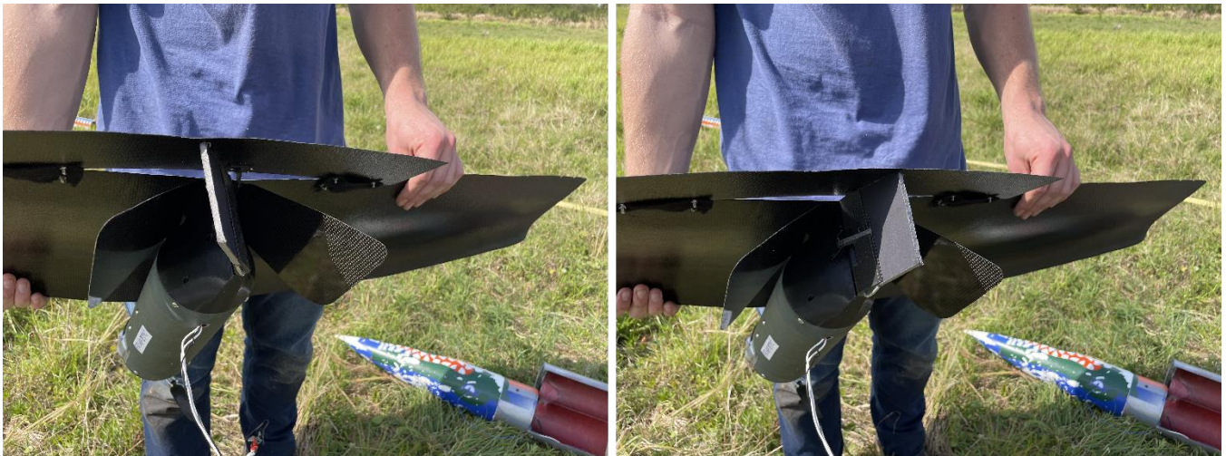
Figure 23: Demonstration of Rudder Function After Flight
