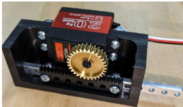
Figure 3: Rack and Pinion Mechanism Assembled
