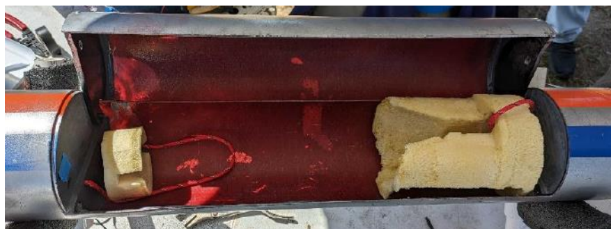
Figure 7: Sabots Attached to Launch Vehicle with Recovery Harnesses
