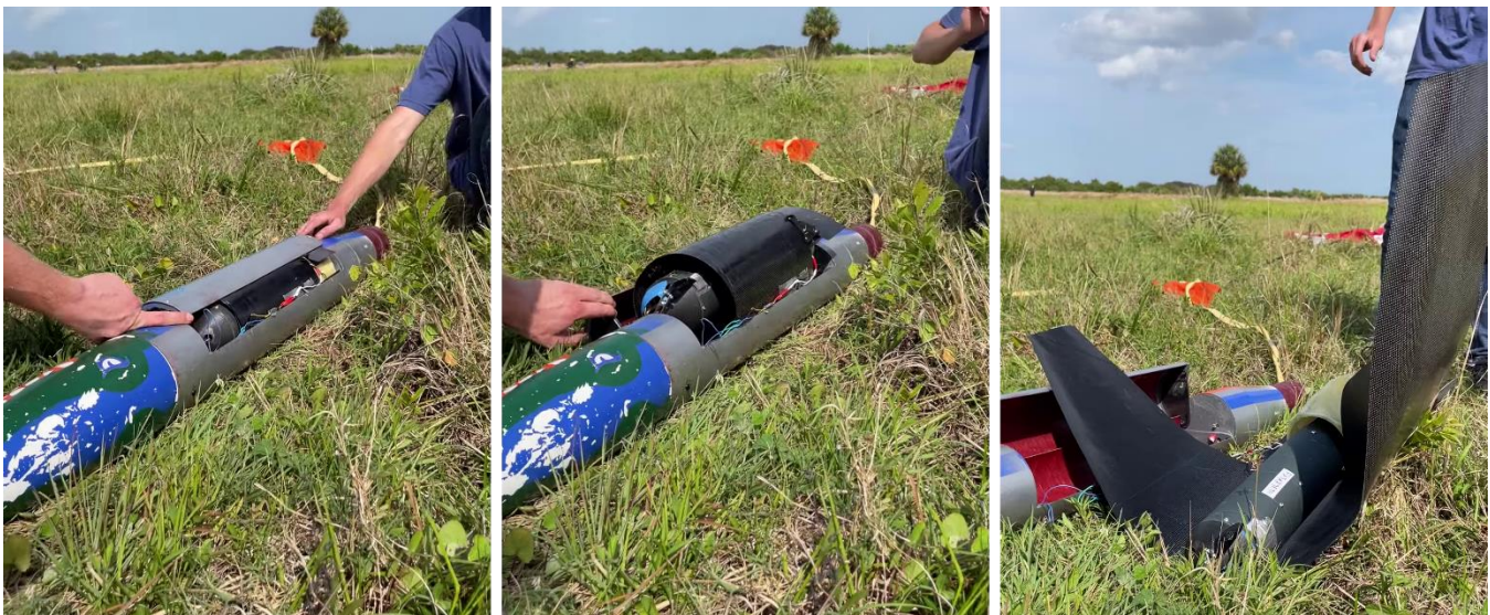
Figure 21: Demonstration of Intended Payload Deployment
