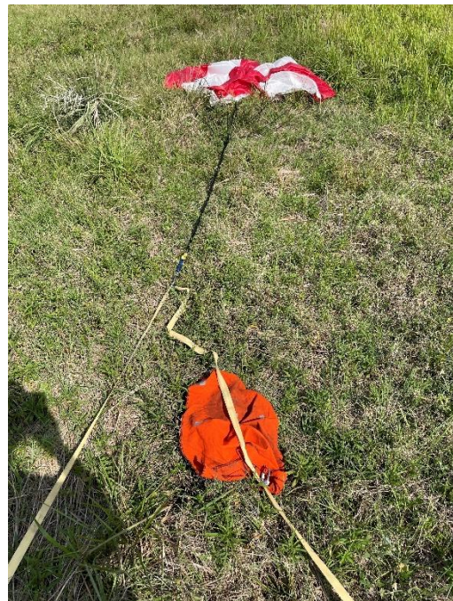
Figure 14: Main Parachute with Parachute Protector
